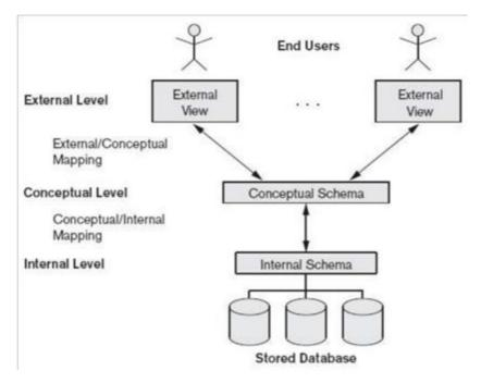
Figure 2.2: The three-schema architecture
