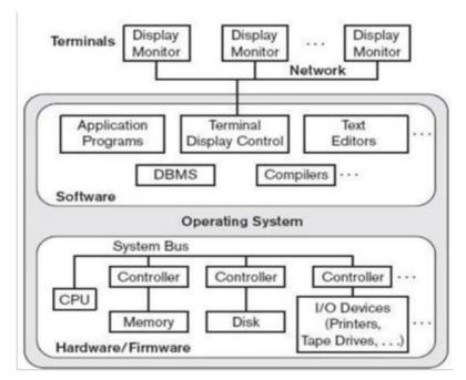
Figure: A physical centralized architecture
