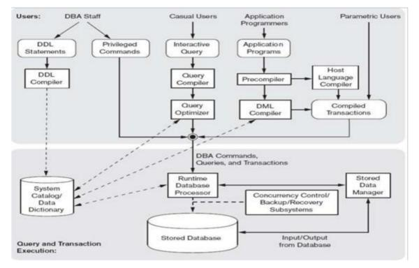
The top part of the figure refers to the various users of the database environment and their interfaces. The lower part shows the internals of the DBMS responsible for storage of data and processing of transactions.
