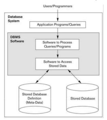
Fig: A simplified database system environment
