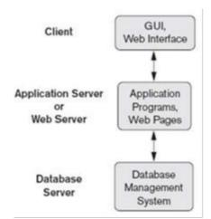
Figure: Logical three-tier client/server architecture
