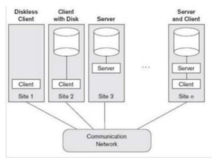
Figure: Physical two-tier client/server architecture
