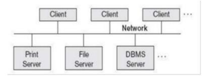
Figure: Logical two-tier client/server architecture
